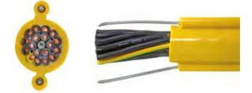
GIFAS KRANFLEX is a special mixture of cold-flexible, weather-resistant PVC acting both as a sheath and as a wire material. The tensile forces that occur are absorbed by two steel cable supporting elements that are arranged in an opposite and axis-parallel manner and which are linked to the exterior sheath.
