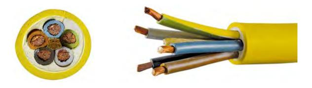
GIFAS PROFLEXX H07 is intended for use in dry, moist and wet spaces or for outdoors use, such as for the connection of equipment in industrial workshops or workshops at risk of fire. In the case of protected, permanent installations, these cables can be operated with a maximum of 1000 V alternating current or 750 V direct current to earth.
