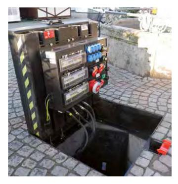
Solid stainless steel construction (V2A/1.4301) 1000x1000mm, load capacity up to 400kN, gas springs for fully automatic opening, shaft cover can be custom-filled, distributor as per the client's request.
